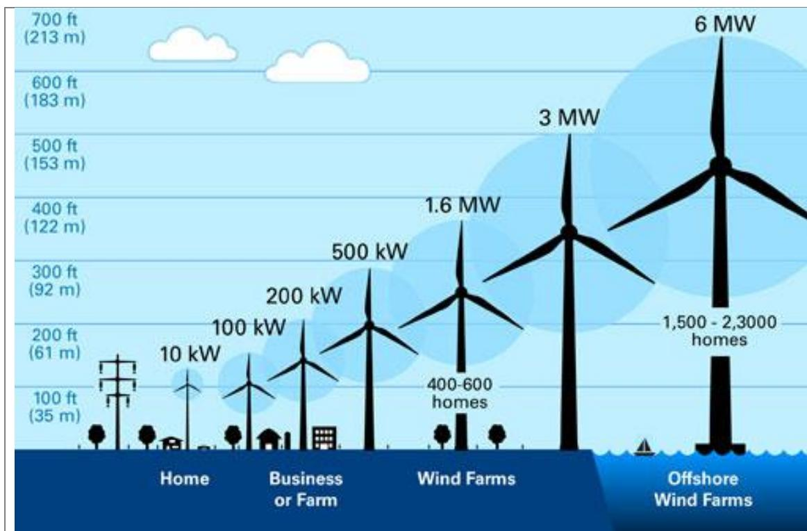
**Figure 3.3.** Wind turbines can be different sizes. The bigger they are, the more electricity they can generate. That’s because winds are stronger the higher you go, and the larger blades can capture more wind. But bigger isn’t always better. Smaller turbines can be best for powering a house or part of a college campus.
