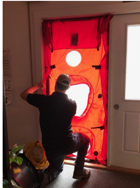
Setting up the blower door test at the Woodford Town Office.
